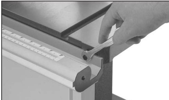
Figure 13. Fastening front fence rail to table.
